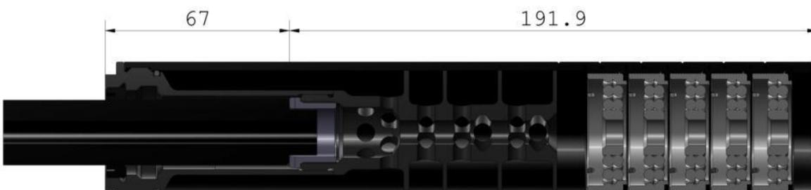
Each additional damping element ( sinter insert holder and sinter insert) is 35 grams and extends the silencer by 15 mm ( 1.5 cm )
